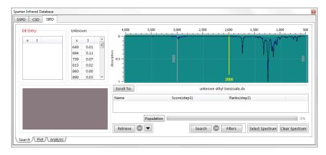
The spectrum has been fit to a Lorentzian function, allowing a set of vibrational frequencies and intensities to be extracted are displayed in the box marked **Unknown:** immediately to the left of the spectrum.\* Features in the unknown spectrum with very low intensity cannot be fit. The fit is shown in black.
