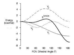
The heavy solid line describes E<sup>torsion</sup> for rotation about the CN bond, while the light solid line, the dashed line and the dotted line correspond to the one-fold, two-fold and three-fold components, respectively. There are two distinct minima.
