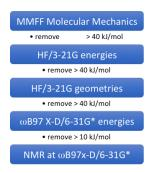
As with the previous protocol, alternative quantum chemical models and energy cutoff values may be substituted for those depicted above. In particular, the B3LYP/6-31G\* density functional model may be substituted for  $\omega$ B97X-D/6-31G\* for both energy and NMR calculations, leading to an additional reduction in computation cost.
