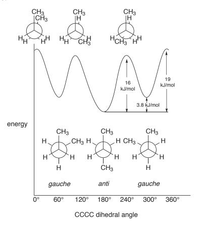
This plot also reveals three energy minima, corresponding to staggered structures, and three energy maxima, corresponding to eclipsed
