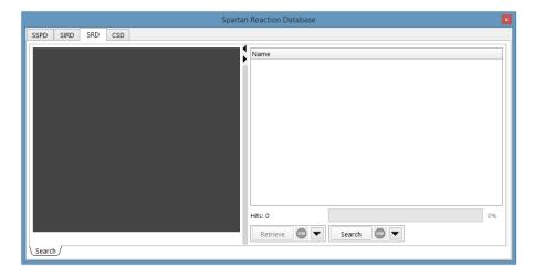
The **SRD** dialog contains a window on the left for previewing structures and a box on the right for listing hits on SRD, as well as buttons at the bottom to control various aspects of the search and subsequent transfer of data into *Spartan*'s file system.
