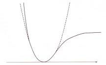
It is possible to extract the harmonic frequency from an experimental spectrum by measuring the spacing of the energy levels associated with the ground and excited states of a particular vibration. (The lines would be evenly spaced were the potential quadratic.) However, such an analysis is impractical for any but diatomic and very simple polyatomic molecules.
