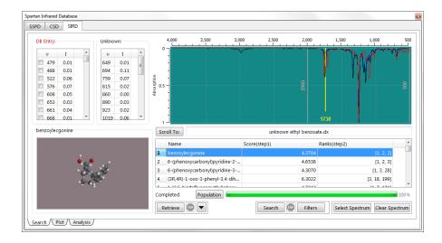
Calculated vibrational frequencies and intensities for the hit are displayed in a box at the top left of the dialog (to the left of the corresponding values for the unknown). *Clicking* inside the box to the left of a (calculated) frequency animates the vibrational motion.
