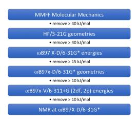
The protocol is fully automated requiring only input of a single conformer and designation of rotatable single bonds and flexible rings. Steps in the protocol may be eliminated, different quantum chemical methods employed and energy filters between steps adjusted. While the protocol has only been thoroughly assessed for <sup>13</sup>C chemical shifts, proton chemical shifts can be added to supplement (or replace) the <sup>13</sup>C data.
