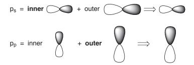
Because the functions in a minimal or split valence basis set are centered on the atoms, they may have difficulty describing electron distributions that fall in between atoms (that is, bonds). *Polarization basis sets* address this problem by providing a set of d-type functions (*polarization functions*) on main-group elements, and (optionally) a
